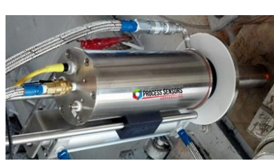
Thermal imager sighted into kiln
