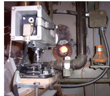
M311, 2-color sensor viewing into burning zone
