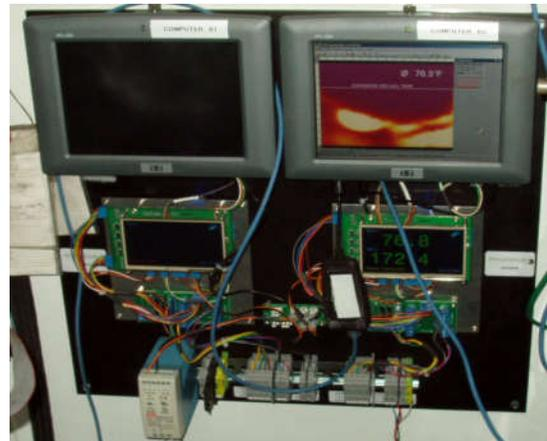
Installation of field PCs for use with Thermal imaging cameras.
