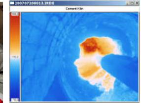
Thermal image of burning zone (Note material dam build-up)
