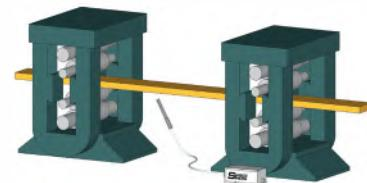
At the **cooling section** of the hot strip mill for determining the cooling curve.
