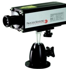
The detector is sensitive to infrared radiation in an area called the “**cone of vision**”. Refer to [Chart 1](#) for the spot size diameter at the shortest, mid-range and longest variable focus distances. The cone of vision/aperture diameter at the optical lens is about **16 mm**. This area has to be kept free from any intervening objects. The spot size diameter for distances not given in the chart can be calculated by interpolation.
