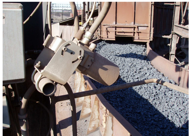
Process Sensors Surveyor Camera Monitoring sintered coke on conveyor. (Arcelor Mittal - Gary Indiana)
