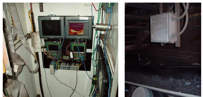
Process Sensors Surveyor Camera Monitoring sintered coke on conveyor. (Arcelor Mittal - Gary Indiana)
