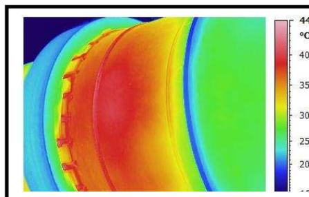
Thermal image of kiln shell hot-spot close to bearing ring at left.
