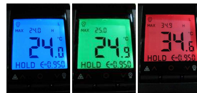
Temperature Display changes color upon Hi/Lo setpoint.
