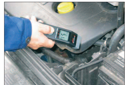
Temperature Display changes color upon Hi/Lo setpoint.
