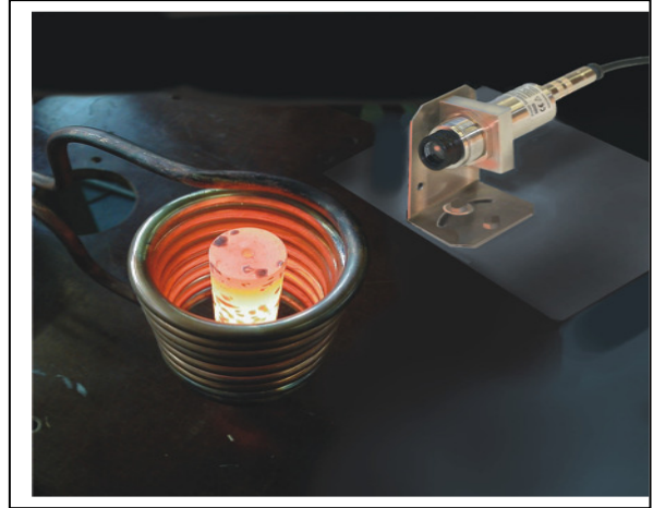
Sirius SI16 pyrometer monitoring induction heated workpiece (File photo)
